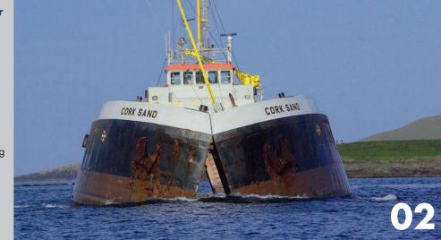
we have a lot of good barges. They have been converted to push barges and are now used in combination with push boats. That makes us more flexible because push boats can be used on other assignments as well. Even so, the split hopper dredgers are very useful and reliable vessels and, after recent overhauls, they also comply with the most stringent standards.'
