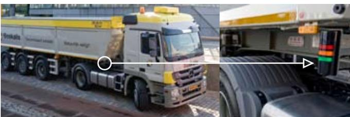
**Boskalis BV has developed a new system to prevent trucks from becoming overloaded. Three lights are installed on the side of the dumper, which are connected to the truck's weighing device. Once the cargo is loaded, the green lights go on and as the loader approaches the critical weight, the lights turn orange. That's when it's time to stop loading. And when the lights turn red, then you know the dumper is overloaded!**
