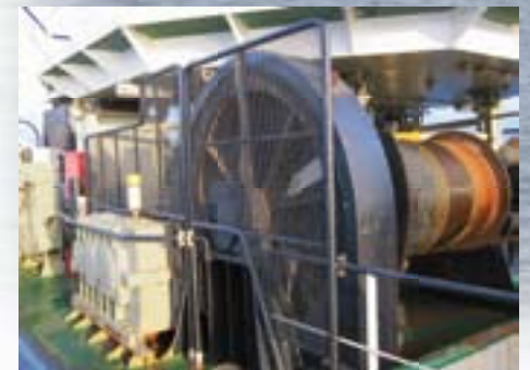
Protective safeguards around deck winches
