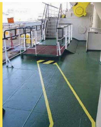
Embarkation platform on Waterway
